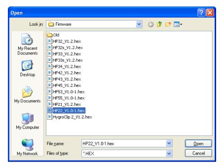
**IMPORTANT**: the HygroLab C1 must be powered during the entire process. Loss of power when the transmitter is being updated may have unexpected results and prevent future operation of the HygroLab C1.
