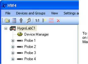
To select the Device Manager for the HygroLab C1, click on it with the left mouse button. HW4 opens the Device Manager form.
